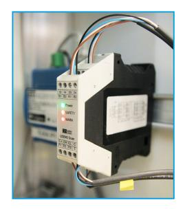
With a total of four relay outputs, the radar Comfort Phantom has an additional relay for the safety field.
